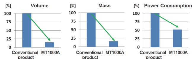
Figure 9 Trends in Reduced Volume, Mass and Power Consumption
