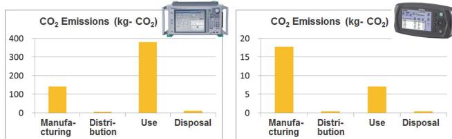
Figure 6 CO<sub>2</sub> Emissions (Left: MP1800A; Right: ML8760A)
