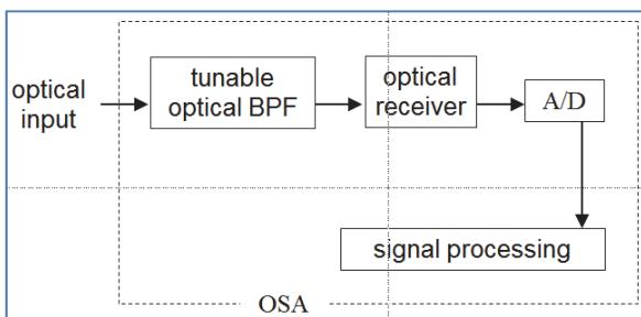
Figure 13 MS9740A basic block diagram
