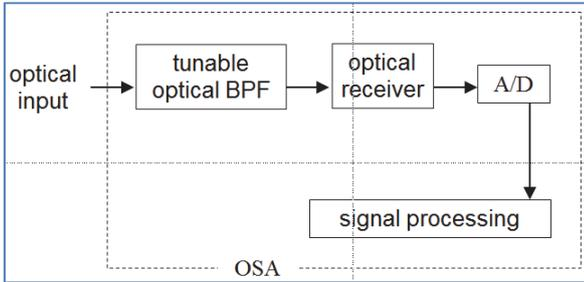
Figure 13 MS9740A basic block diagram
