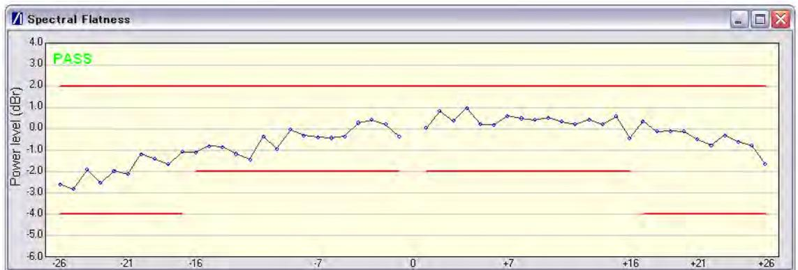
**Figure 11-31.** [Spectral Flatness] Window: Example for 20 MHz Non-HT
