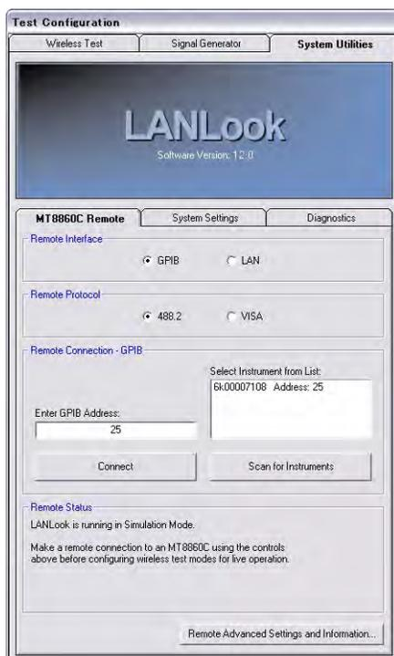
**Figure 5-1.** [System Utilities] Tab for GPIB
