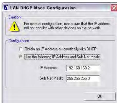
**Figure I-48.** LAN DHCP Mode Configuration
