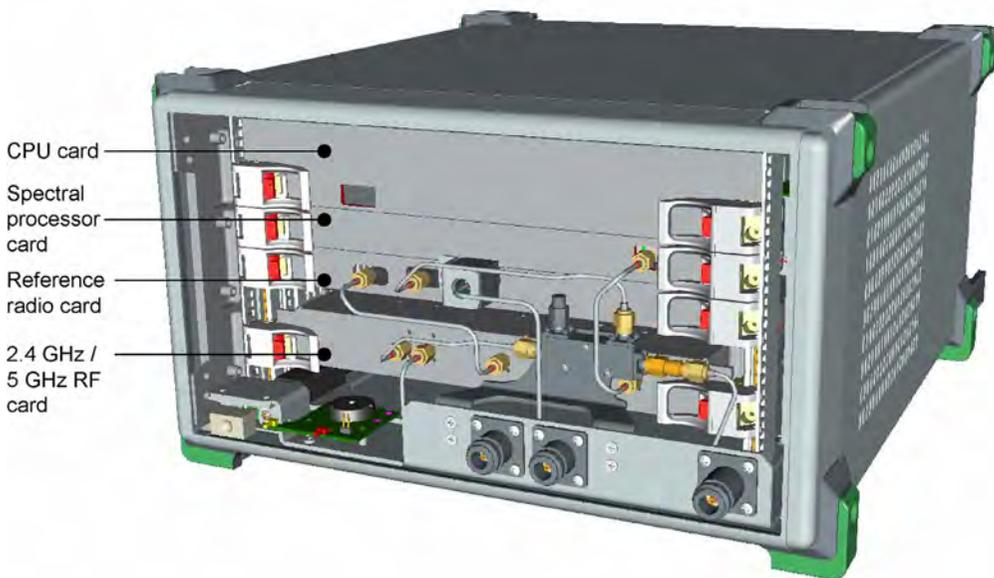
**Figure 1-3.** MT8860C Internal Structure
