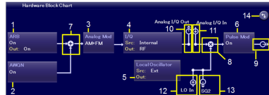
Hardware Block Chart (explanation)
