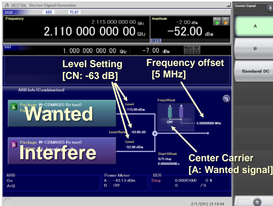
MG3710A Settings for Wanted Signal + Modulated Interference Signal
