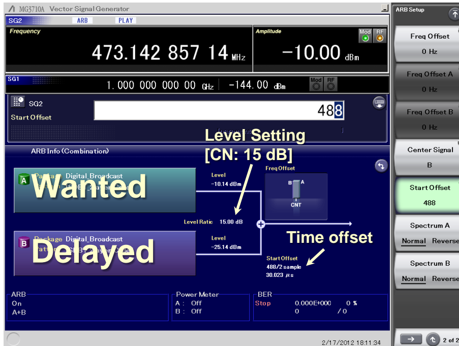
MG3710A Settings for Wanted Signal + Delayed Signal
